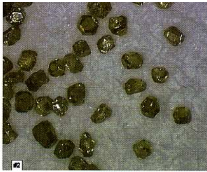
Black & Decker's metallurgical lab conducts a variety of tests that include the analysis of steel alloy and powder-metal gears, thickness checks of titanium and zinc plating, and carbide analysis. In this test, the laboratory tested the diamonds used in a diamond tile cutting blade. Shown here is a micrograph of diamonds (left) and a processed image used for extracting statistical data (right). Photo: Clemex Technologies
