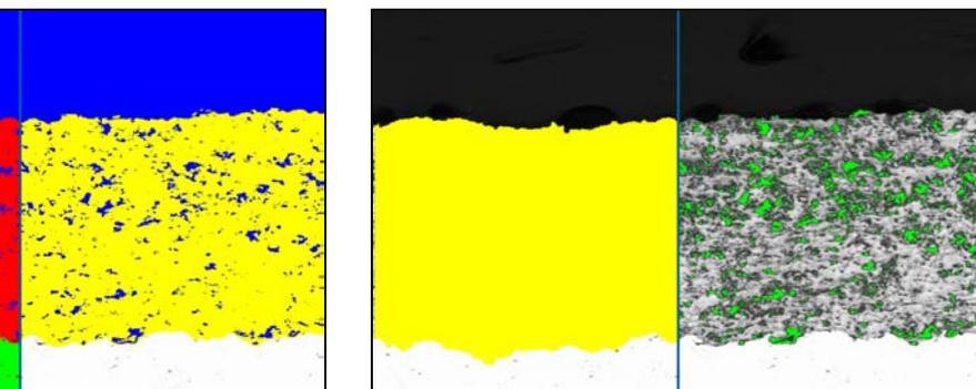
**Figure 1b:** Binary operations remove inclusions and dust particles from the coating.
