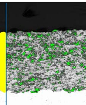
**Figure 2b:** Porosity (green) isolated from the blue detection using a *Boolean* operation.
