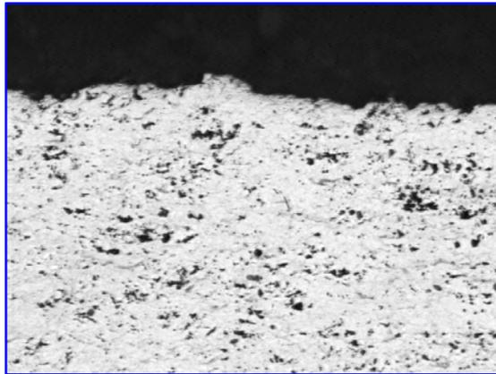
Characterization of a Thermal Spray Coating
