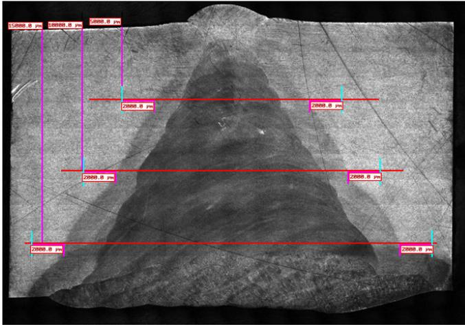
**Fig. 3:** Step 1: Straight lines drawn to determine depth. Step 2: Red lines indicate the traverses' paths. Step 3: Distance of 2000.0 microns from the edge of the heat affected zone into the base material. Step 4: Cyan lines drawn to indicate the beginning and the end of each traverse.
