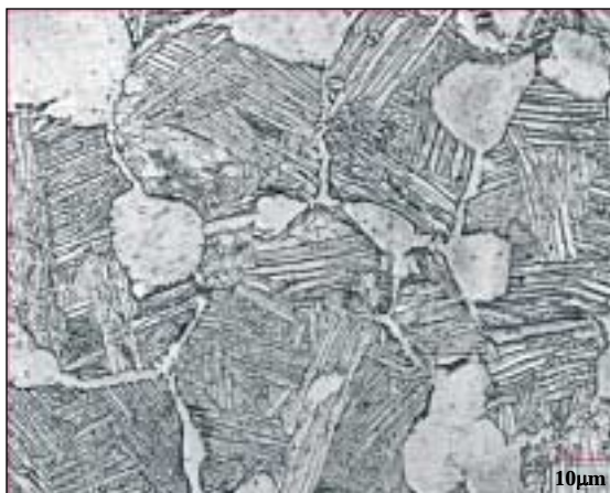
Fig. 8 — Fine lamellar alpha titanium microstructure is shown at 500X magnification after the Multilayer Grab was executed.
