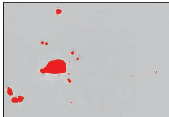
Grey Threshold on reconstructed image. Large and small particles are in focus.
