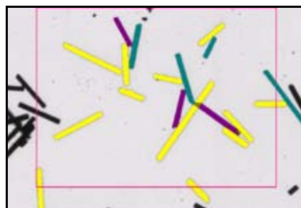
Guard frame (red) implemented and long objects with ID points outside the guard Frame are rejected.
