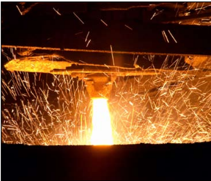
Dumping slag in fusion
