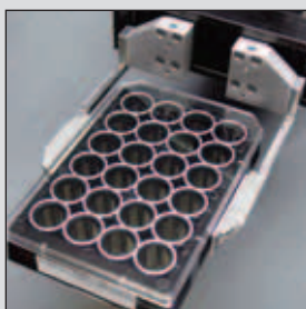
System can accommodate all standard sized microplates.
