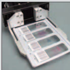
Robotic hand holds up to 4 slides at once
