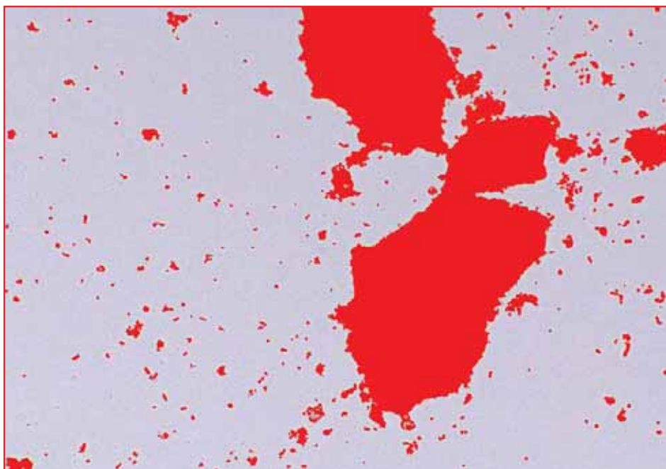
Figure 2: Particles as detected into the red bitplane using automatic gray thresholding.
