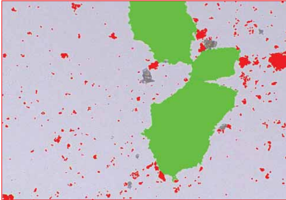
Figure 3: Features thinner than 10 microns and those with holes inside were eliminated. Yellowish particles were isolated into the green bitplane for separate measurements.
