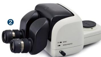
2 P2-TERG50 Trinocular Tilting Tube (eyepiece: port 100:0/50:50)
